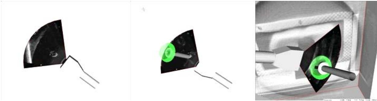
Figure 4. Left: US image of tool shaft; Center: US image with virtual tool added. Right: US and tool augmented by 3D CT of phantom and target (dark disk on PVA-C is the “valve orifice”).
