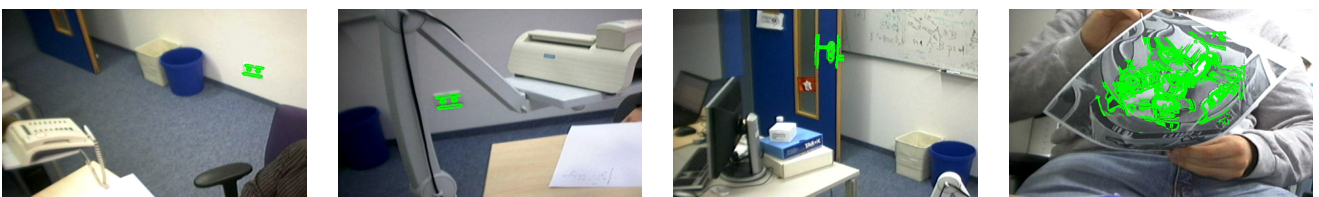
Figure 9. Patch 3D orientation estimation. Like Gepard [8], DOT can detect planar patches and provide an estimate of their orientations. DOT is however much more reliable as it does not rely on feature point detection, but parses the image instead. The corresponding video is available on http://campar.in.tum.de/Main/StefanHinterstoisser .
