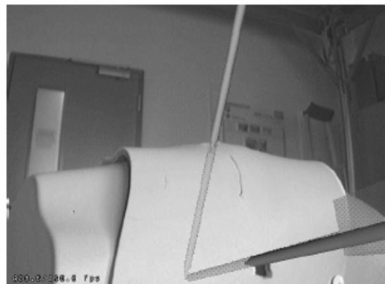
Fig. 5b: After tracking the chest model by infrared markers and an external camera system, ports and instruments are projected upon the surface of the chest model to determine the calculated incisions for port placement.
