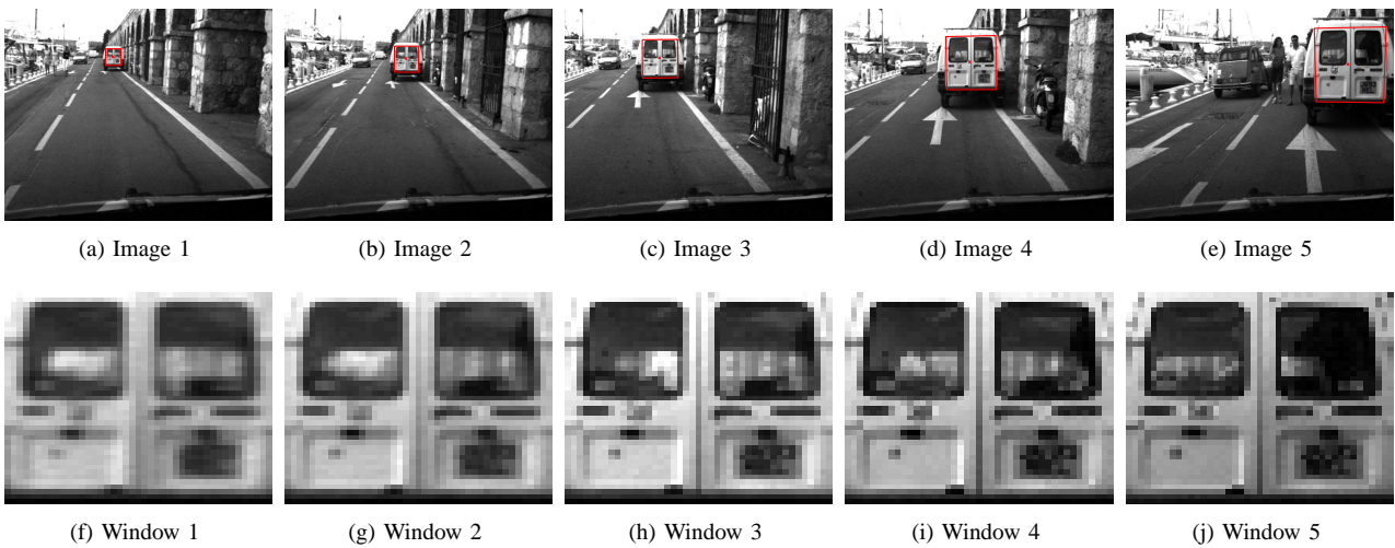
Fig. 5. Tracking a template on the back of a car.
