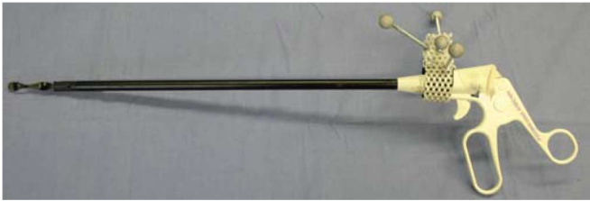
Fig. 10. The endoscopic surgical instrument is tracked by the external optical tracking system and has to be guided to the target spots.
