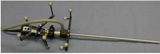
Fig. 5. The laparoscopic camera consisting of two marker targets tracked by the optical outside-in tracking system.
