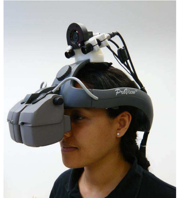
Fig. 4. The used video see-through head mounted display [51] consists of two color cameras simulating the eye's view and an infrared camera for inside–out tracking.
