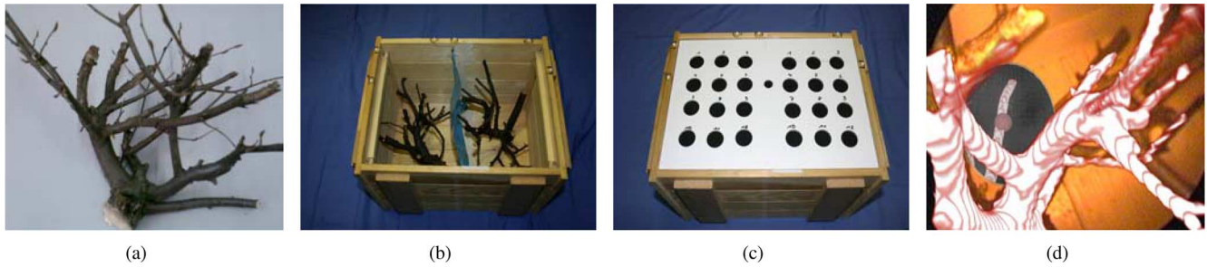
Fig. 14. Two wooden branches are installed on the bottom of the box and visually separated by a plastic foil. For the experiment the box was closed with a plane having twelve ports to each branch.
