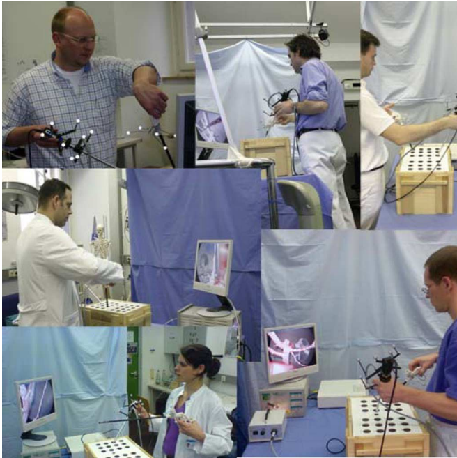
Fig. 13. Six of 12 surgeons of our clinical partner guide the surgical instrument inside the phantom using the video images of the laparoscopic camera presented on a monitor.
