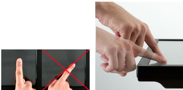
(a) Yaw: finger parallel to the vertical edge of the display (b) Pitch: finger between 15 and 60 degrees
