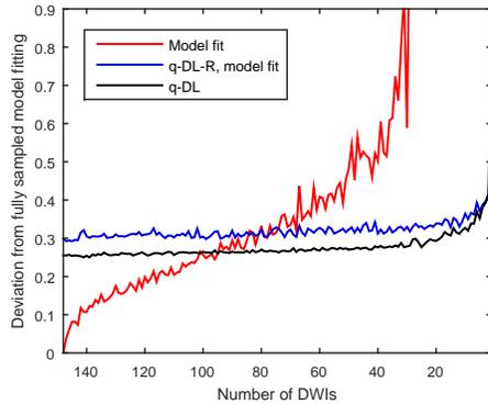
**Fig. 2.** Error evaluation of different methods at different acceleration factors. Root-mean-square deviation from the radial kurtosis estimated by the standard pipeline (fully sampled model fitting) is used as error metric. Model fitting is outperformed by the proposed methods when less than 70 DWIs are used.
