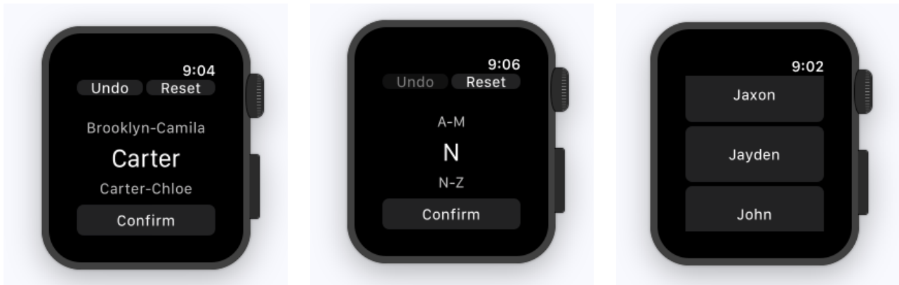
Figure 2: Screenshots from the watch simulator showing the three possible interface modes: (a) shows the binary search, (b) the hybrid mode and (c) the linear search.
