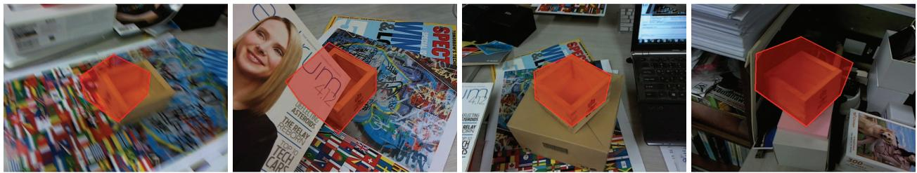
Fig. 12. Tracking failure cases. **Left:** Fast motion, **Middle-Left:** Heavy occlusion, **Middle-Right:** Similar object and background color, **Right:** Low contrast by poor illumination.
