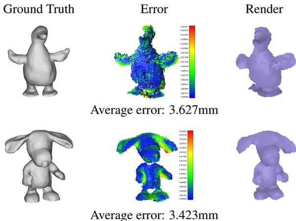
Figure 8. Non-rigid reconstruction of the *Duck* and *Snoopy* sequences from the KillingFusion dataset [27]. Our method reconstructs the sequences with a smaller error margin.
