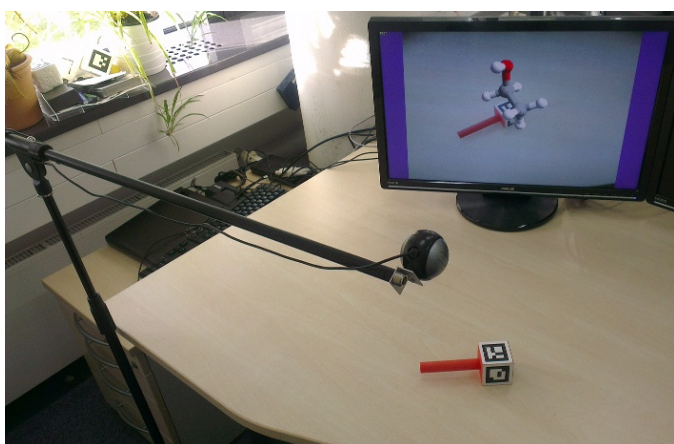
Fig. 3. Computer setup for the Augmented Chemical Reactions application, using a webcam a physical cube on a handle and a monitor. The keyboard that is required to cycle through a set of molecules is not shown.
