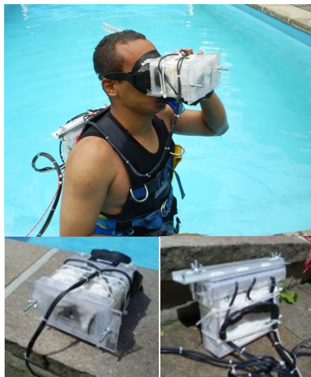
Fig 4. Hardware configuration of the UWAR system used in the experiments. (Top) Diver wearing the UWAR system. (Left-Bottom) Watertight housing for Logitech Quickcam Pro 4000 and eMagin Z800 3D Visor HMD. (Right-bottom) HMD driver and umbilical connections to surface.
