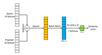
Figure 5. Our proposed Query-guided Similarity Network (QSim-Net). QSimNet introduces a simple query-guided net to estimate the similarity between the query and the gallery image. This is learned end-to-end with the rest of the network.
