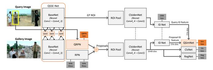
Figure 2. Our proposed QEEPS network architecture. We pair the reference OIM [37] *bottom network* with a novel Siamese *top network*, to process the query and guide the person search at different levels of supervision (cf. Sec. 4). The novel query-guidance blocks of our approach, displayed in orange, are trained end-to-end with the whole network with specific loss functions (*darker orange boxes*).
