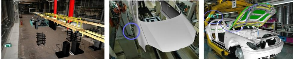
Figure 1: Industrial AR: (a) Change management in factory planning, (b) Interfering edge analysis, (c) Head space in assembly
