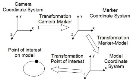
Figure 3: Accuracy chain for 3D measuring
