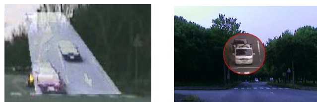
(a) Virtual slope revealing occluded objects in the opposite lane of intersection (Taya et al., 2005)
