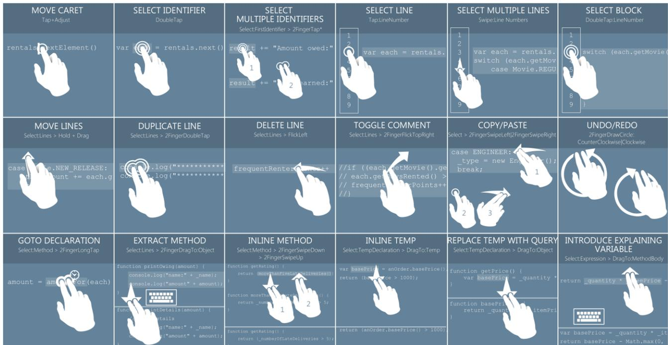
Figure 4: Gesture set for basic selection, editing and refactoring operations for text-based editors on touchscreens. (*SelectFirstIdentifier > 2FingerTap \** means: Select the first identifier, then (>) perform multiple (\*) taps using 2 fingers.)
