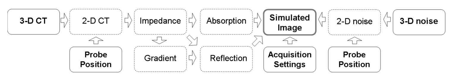
Above: simulation pipeline, from 3-D CT data, 3-D noise, probe position, and acquisition settings an US image is simulated. Right: setup with haptic input device (Phantom Omni).
