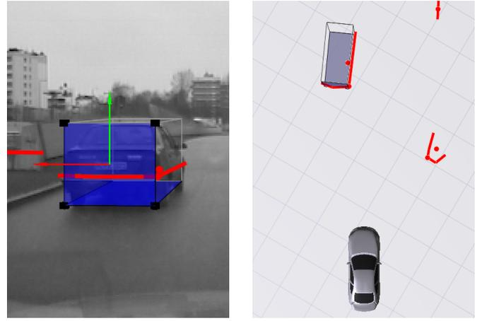
Figure 3. Reference object (blue cuboid) with actual 3D position set from laser scanner measurements (red).
