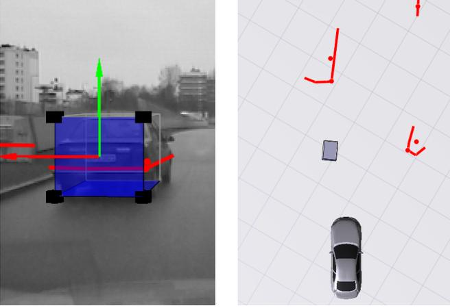
Figure 2. Reference object (blue cuboid) extracted from the camera image only; laser scanner data is shown in red color.
