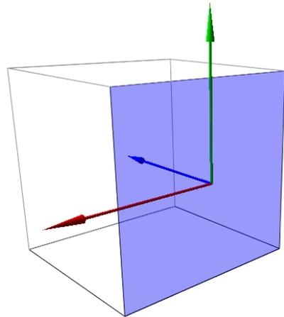
Figure 1. Cubic model of a reference object with orientation vector (blue arrow) and its face towards the imaging sensor (blue face).
