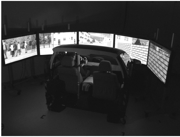
Figure 2: Static driving simulator with plasma screens and mock-up
