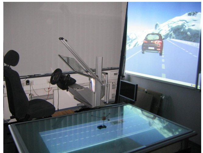
Figure 3. The Setup in the Laboratory: The Table-top Environment in Front of a Driving Simulator
