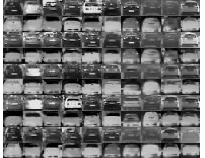
Fig. 3. Small subset of the vehicle training set. Grey-scale training samples are in odd rows. Even rows contain the corresponding FIR samples.
