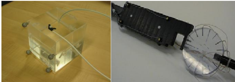
Figure 2: Hybrid tools with both electromagnetic sensors and optical markers (adopted from [FIS05b]) and [CHU04]
