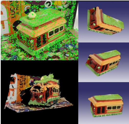
Figure 2: Steps of the reconstruction process. SIFT features are used to match images (upper left), a dense point cloud is reconstructed from matching points (bottom left), finally a textured mesh is produced (right).
