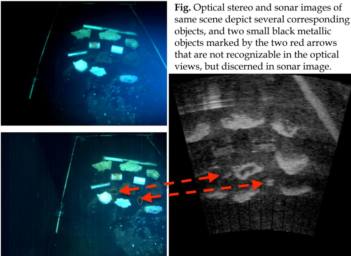
**Fig.** Optical stereo and sonar images of same scene depict several corresponding objects, and two small black metallic objects marked by the two red arrows that are not recognizable in the optical views, but discerned in sonar image.
