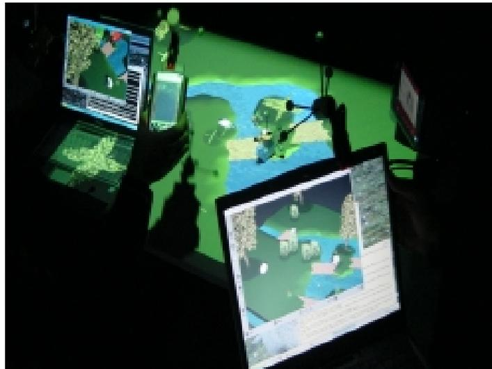
Figure 1.1: The *Shared Environment Entertainment Pasture* is an experimental system to test interaction techniques with AR. It is based on a virtual landscape with sheeps projected onto a table and where the landscape also can be seen through laptop screens, PDAs and HMDs. Courtesy of the SHEEP team, <http://campar.in.tum.de/Chair/ProjectSheep>
