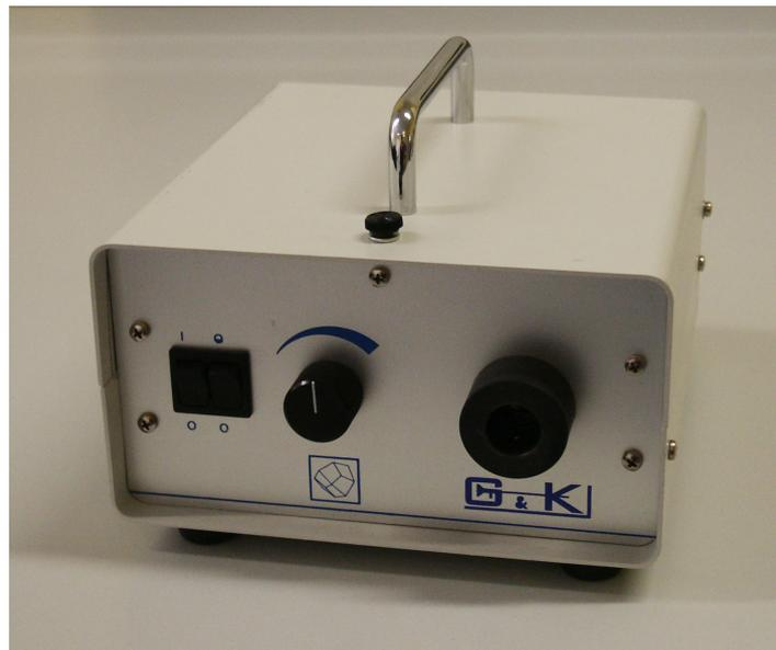
Figure 6.1: The source of distortion for experiment 1.3 was the light source of an endoscope.
