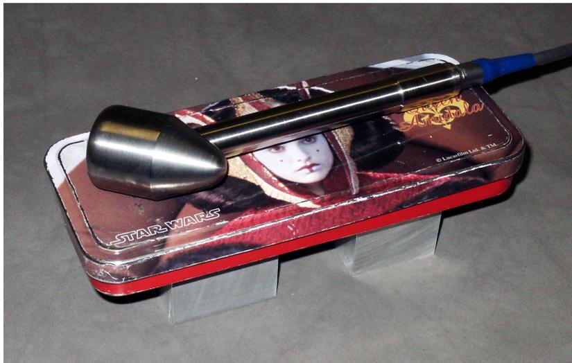
Figure 7.3: The source of distortion for trial 1 of experiment 2.5. It is composed of two lead blocks, a pencilbox and a gamma probe.
