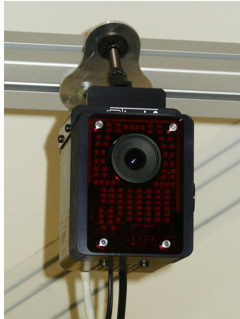
Figure 5.4: The picture shows one camera, model ARTtrack2, manufactured by Advanced Realtime Tracking GmbH.
