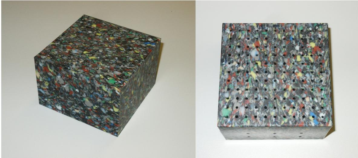
Figure 3.3: The polymer block used by Kaur for one approach of distortion correction for electromagnetic tracking. Picture taken by Kaur.
