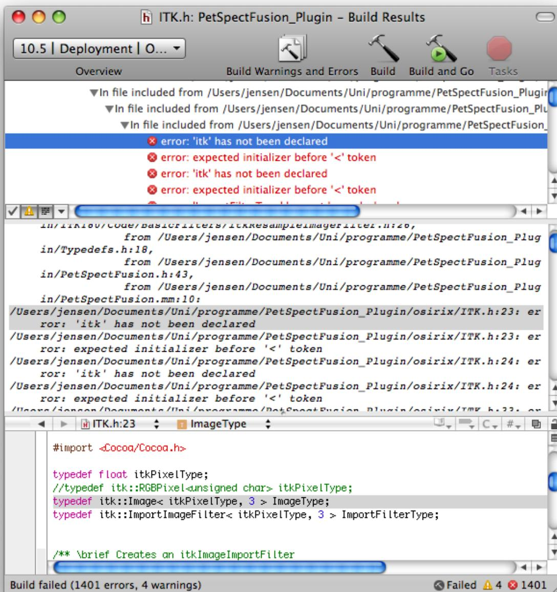
Figure 11: This error was caused by incorrect path settings. The compiler included an OsiriX header instead of an ITK because both them have the same name.
