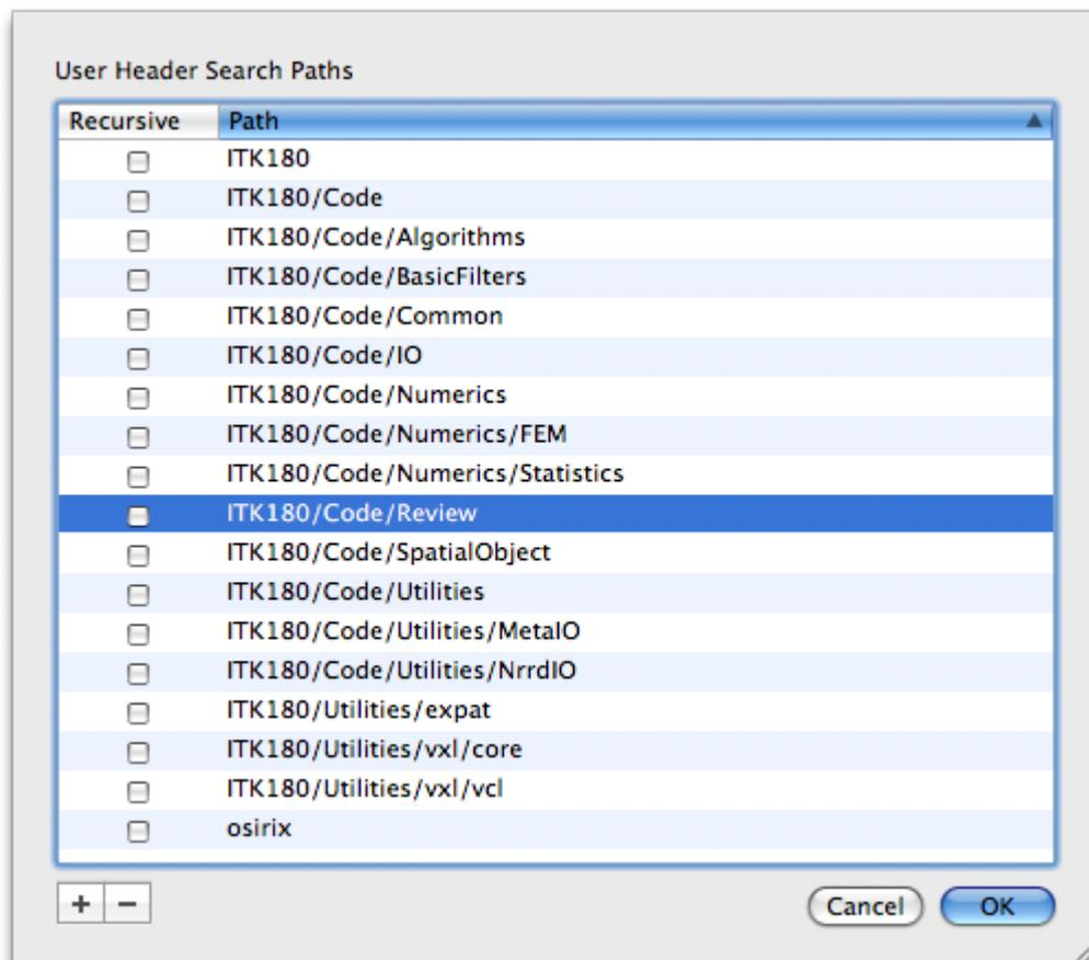
Figure 2: The user header search paths. It is extremely important that the ITK paths are located before the OsiriX path because certain files in OsiriX and ITK have identical names aside from their capitalization and HFS+ is per default not case sensitive.
