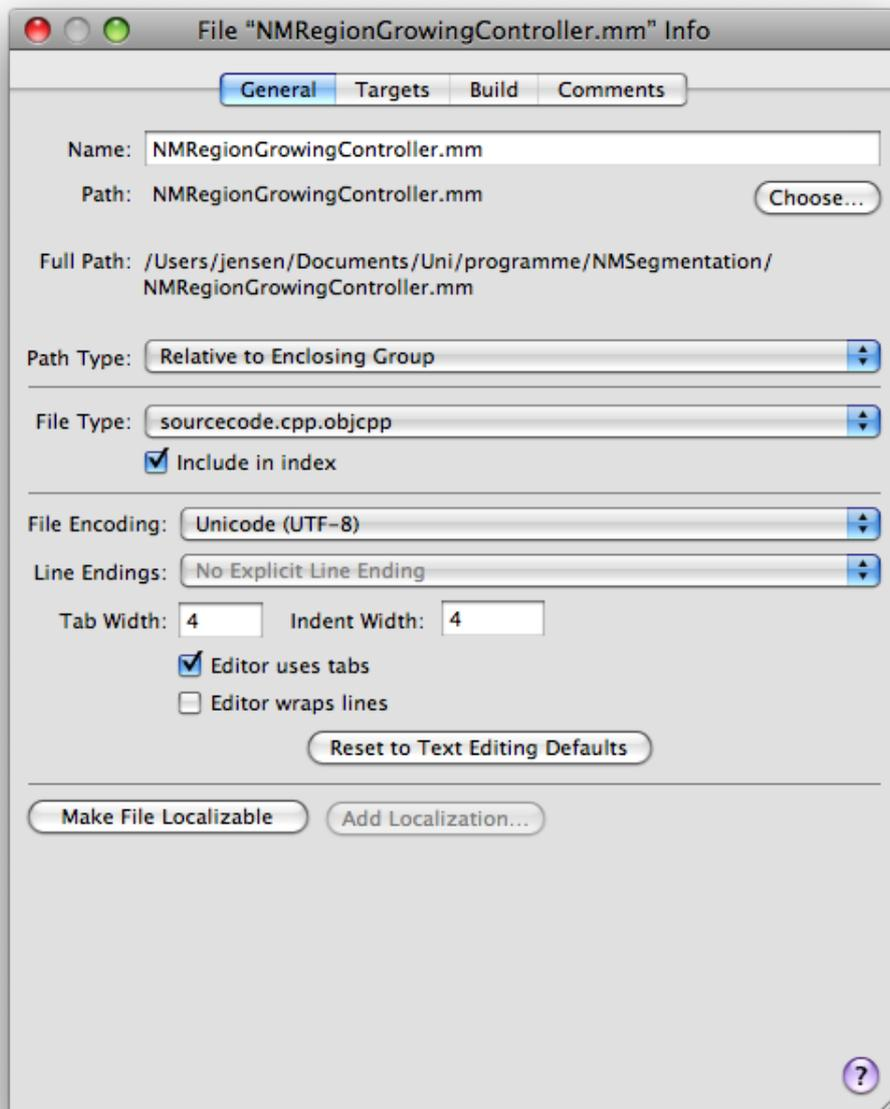
Figure 10: The file info dialog. If your classes uses C++ code make sure its file type is marked as can be seen in this figure.
