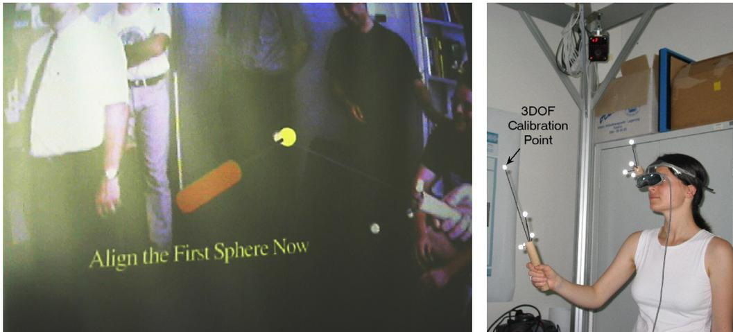
Figure 1.6: HMD calibration with a pointing device
