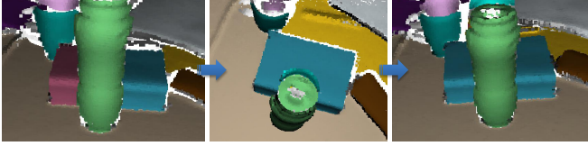
Fig. 5. Benefits of the proposed Segment Merging procedure: an object initially segmented into two parts due to an occluding foreground surface (left), is then merged into the same segment when a different camera view reveals the right connectivity (middle and right)
