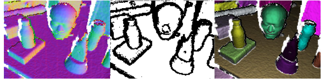
Fig. 3. Normal map (left), normal and geometrical edge map (middle) and resulting depth map segmentation with shading (right)
