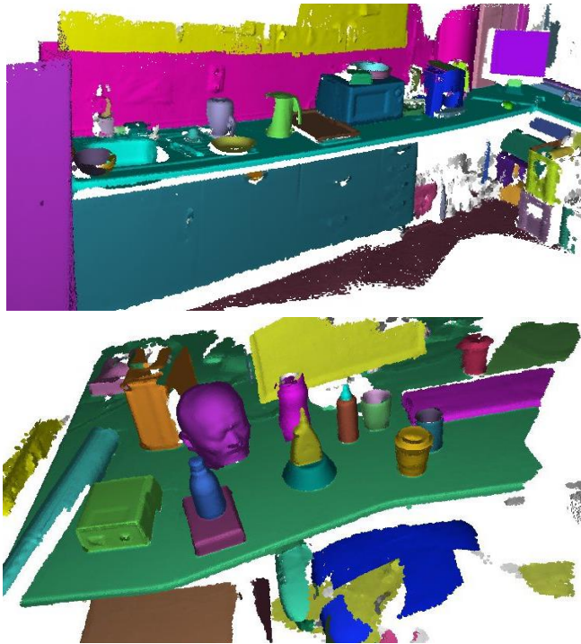
Fig. 1. Real-time incremental segmentation applied to the reconstruction of a kitchen (top) and a table-top scene (bottom). As witnessed by these examples, the proposed segmentation method can adapt to different scenarios and can yield accurate segmentation since it applies to scenes reconstructed by merging multiple views via SLAM, this usually providing more consistent, reliable and meaningful segments than the single-view case.
