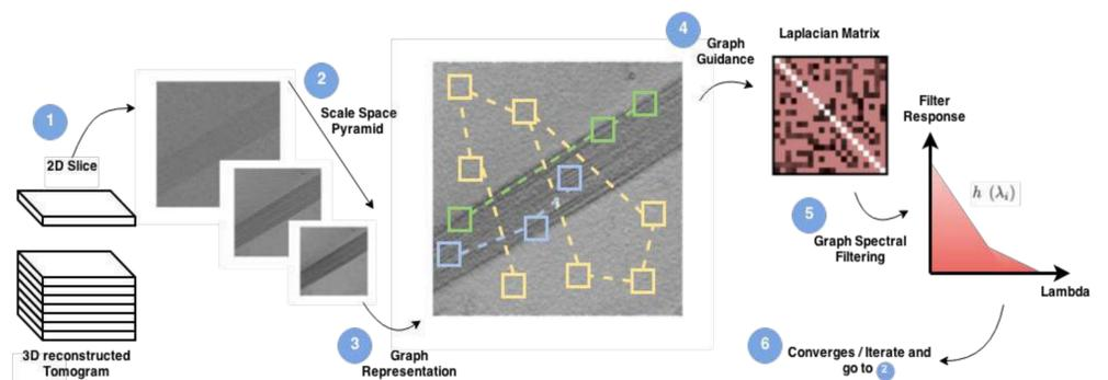
**Figure 1: MG<sup>2</sup>F Framework:** A noisy image slice from the 3D reconstructed tomogram is fed to the algorithm, where the graph is built on a selected scale space image (i.e. coarse grid) acting as a guidance for the regularized graph spectral filter.
