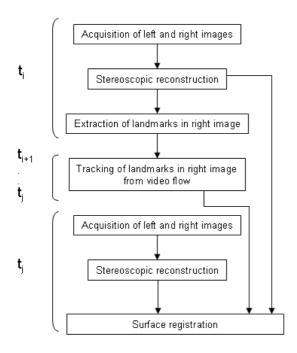
Figure 1: Image acquisition and registration workflow
