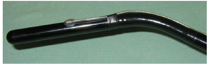
Fig. 3. Electromagnetic sensor coil glued to the tip of a flexible laparoscopic ultrasound transducer in order to determine the position and orientation of the ultrasound B-scan plane of the transducer.
