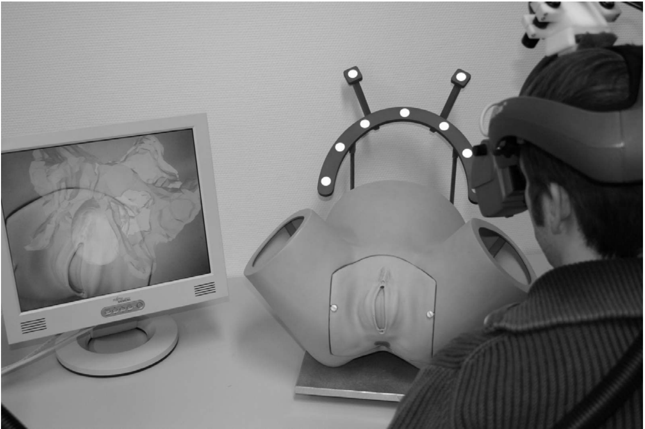
Figure 1. The AR delivery simulator setup; user working with human delivery system[14] wearing the RAMP HMD system.
