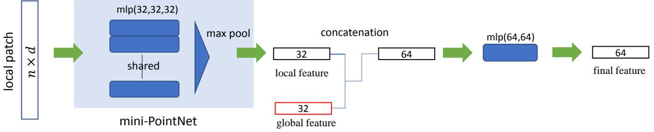
Figure 10. Pipeline for processing a single local patch.
