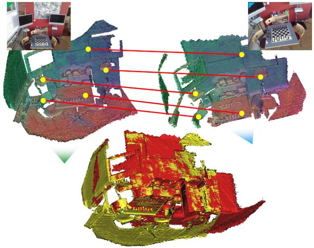
Figure 1. *PPFNet* generates repeatable, discriminative descriptors and can discover the correspondences simultaneously given a pair of fragments. Point sets are colored by a low dimensional embedding of the local feature for visualization. 3D data and the illustrative image are taken from 7-scenes dataset [39].
