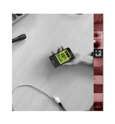
During the registration of the mobile phones, a visual representation of each phone is generated on the surface at the position of the corresponding phone.
