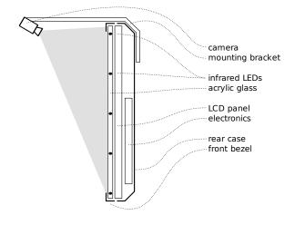
Figure 4. Schematic view (not to scale)
