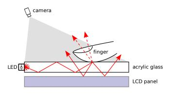
Figure 3. Inverted FTIR
