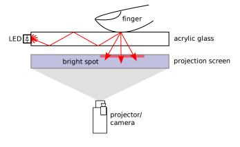
Figure 2. FTIR principle of operation
