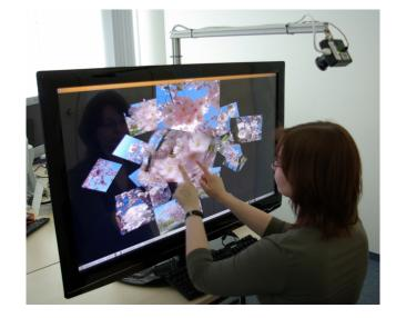
Figure 1. Using an LCD screen with inverted FTIR
