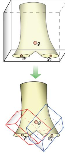
Fig. 2: Generation of child VOIs. Each child VOI is oriented along the line from a detected furcation point  $g$  to the center of gravity  $g_i$  of child branches. Width and height of a child VOI are set to be twice as large as the radius of the child branch.
