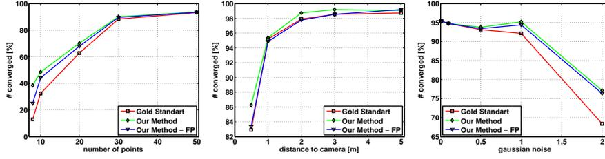
Figure 4: Convergence rate in percent; the first graph shows results with an increasing number of points and a Gaussian noise of 0.5; the second graph shows the effect of an increasing distance from the scene with 50 points and a Gaussian noise of 0.5; the last graph shows the results with 50 points and varying Gaussian noise from 0.01 to 2; it shows that the additional intensity information enables our approach to be more robust even with a fronto-parallel assumption (FP).
