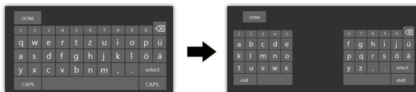
Figure 5: The keyboard layout was changed for the UI with the classical interaction technique. The keys were arranged differently (alphabetic layout).
