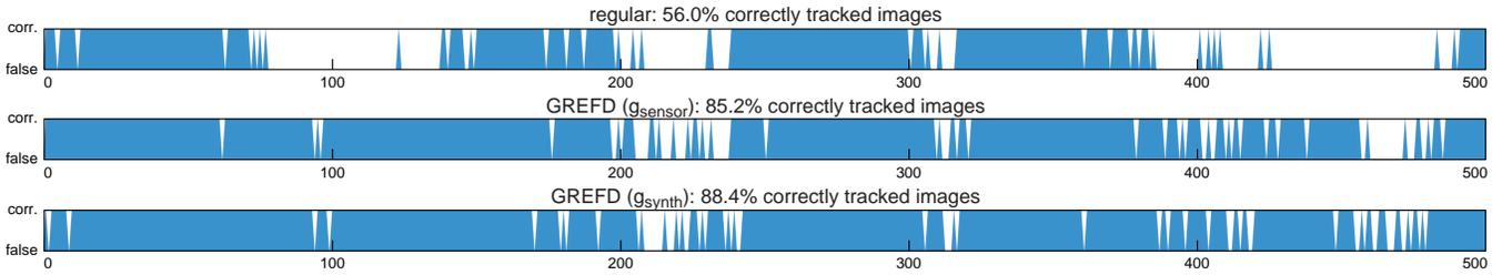
Figure 3: Distribution of correctly tracked images in a sequence of 500 frames showing the “Isetta” template using regular feature descriptors, real gravity measurements in GREFD( $\mathbf{g}_{sensor}$ ) and the proposed method in GREFD( $\mathbf{g}_{synth}$ ). The latter two methods provide comparable results.
