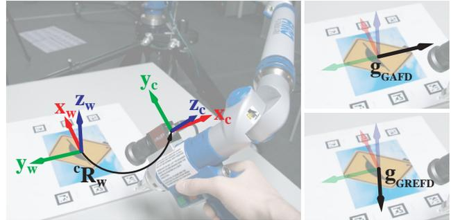
Figure 4: Visualization of the involved coordinate systems and the synthesized gravity vectors for the evaluation of GAFD and GREFD.
