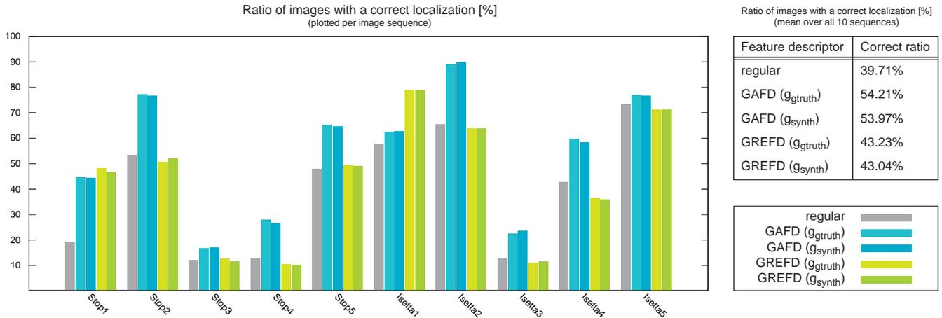
Figure 6: Results comparing GAFD and GREFD with regular rotation-invariant local feature descriptors. While GAFD outperforms regular descriptors for virtually all sequences, the performance of GREFD is strongly depending on the steepness of the camera angles used.
