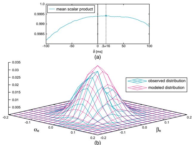
Figure 2: Correlation between the measured and the ground truth gravity vectors as a function of the delay between the two (a). The observed error distribution of the real gravity measurements can be modeled with a Gaussian distribution (b).
