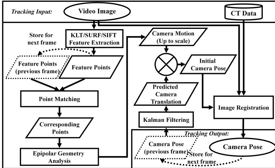
Fig. 1: Processing flowchart of our motion tracking method.
