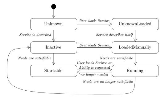
Figure 3.8: Stages in the service life cycle
