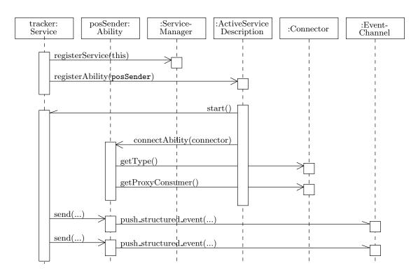
Figure 5.5: Interaction between a DWARF Service and the middleware.
