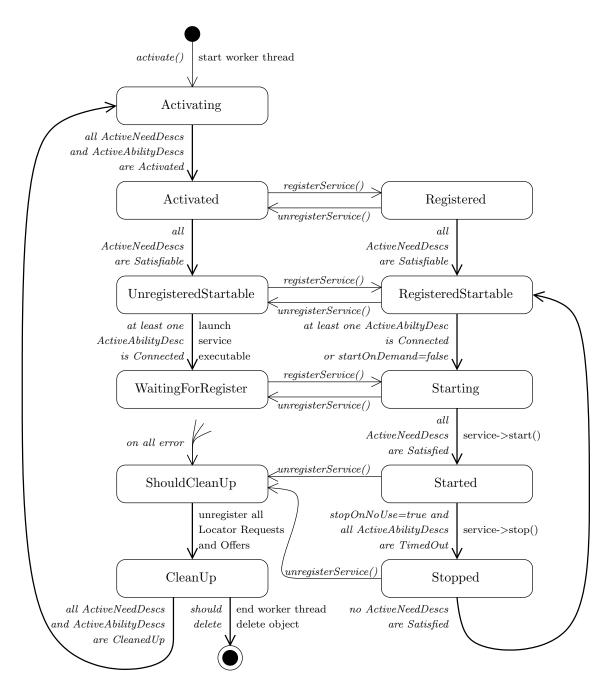
Figure A.1: State diagram for the ActiveServiceDescription\_i class.
