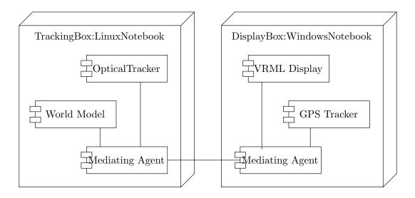
Figure 5.1: Deployment of Distributed Mediating Agents. Each network node has its own Mediating Agent. The DWARF Services communicate locally with the Mediating Agents, which handle network communication. Compare this to Figure 3.1 on page 30.
