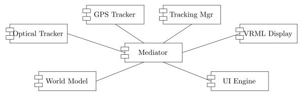
Figure 3.1: The mediator pattern in DWARF.
