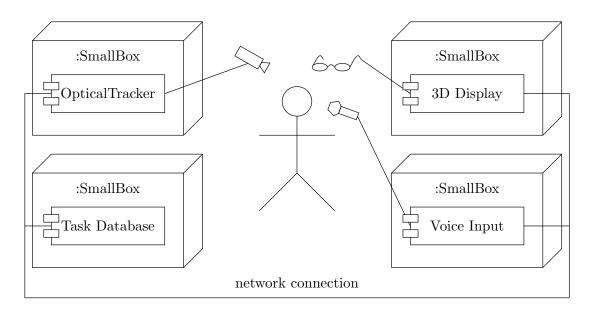
Figure 2.3: An Augmented Reality system based on cooperating components. The user carries several small hardware components with him, each with its own devices attached. They are configured to cooperate.
