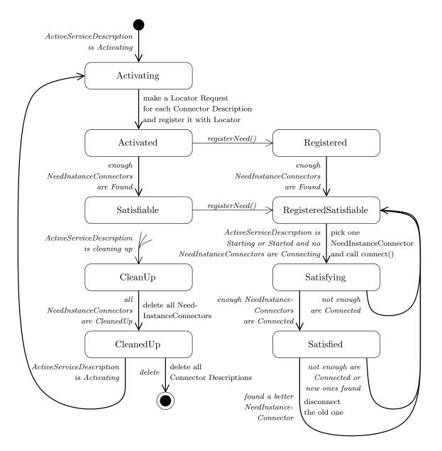
Figure A.2: State diagram for the ActiveNeedDescription\_i class.
