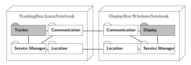
Figure 5.2: Subsystems of the DWARF middleware.
