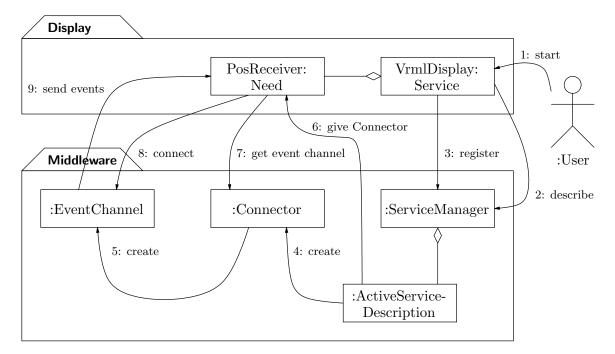
Figure 3.6: Example interaction between a display Service and the middleware
