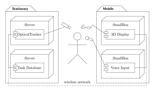
Figure 2.4: An Augmented Reality system based on self-assembling cooperating Services. The user is carrying two small wearable computers with him, and these cooperate with stationary ones in the room he is in. This figure represents one possible configuration of the system. As the user walks on, the mobile systems could disconnect from the database and connect to other tracking devices.
