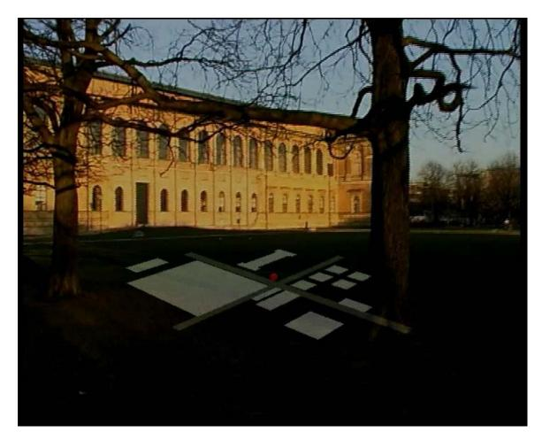
Figure 7.3: User's view of outdoor navigation with the DWARF demo system. A three-dimensional map is superimposed on the user's field of view. Note that the building ahead is also directly ahead on the map, since the map is oriented as the user is.
