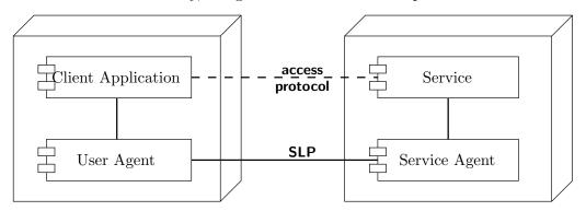
Figure 4.1: Deployment of SLP subsystems without Directory Agents
