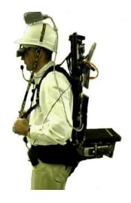
Figure 7.1: A side view of our prototype wearable computer built with DWARF. Note that two laptops are used, and that there are no trailing cables. The display on the lower laptop was kept open so that the user's view could be shown to an audience as well.
