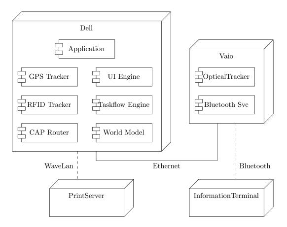
Figure 7.2: Deployment of the DWARF Services in the demonstration system
