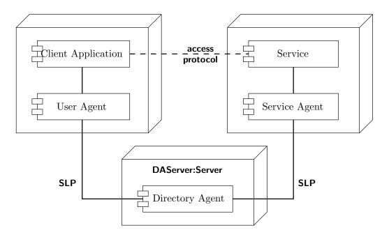
Figure 4.2: Deployment of SLP subsystems with Directory Agents
