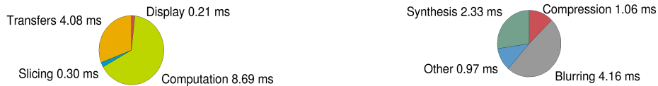
Figure 2: Timing overview (left) and a breakdown of the “Computation” step on GPU (right).
