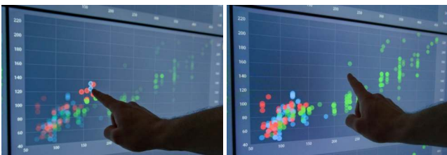
Figure 9: Users can exclude selected items with a fling gesture. The user starts a fling gesture on the currently selected items (left). The selected items are filtered out. Since all selected items vanished, no selection is active anymore and all elements are displayed with the usual transparency again (right).
