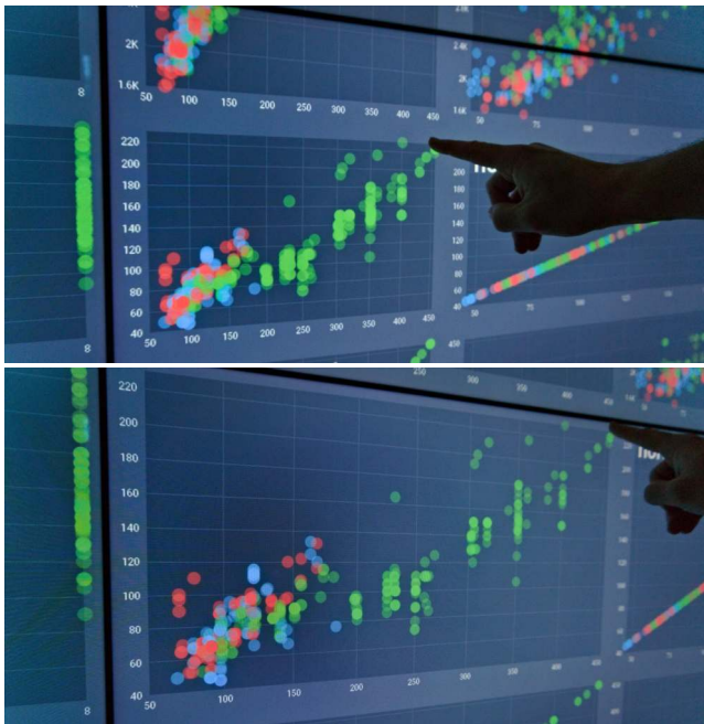
Figure 4: Global F+C by directly resizing a plot. (top) The user long-taps on the corner of the plot to initiate a horizontal and vertical resize. (bottom) The plot corner moves along with the finger and therefore the plot expands. The plots to the right and top shrink accordingly.
