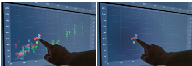
Figure 8: A long-tap gesture on selected items filters out the non-selected ones. The user initiates filtering by tapping the currently selected items (left). After a fixed duration, a long tap is detected. The filtering takes place and all other items disappear (right).
