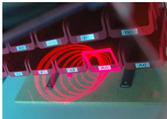
Figure 12 Tunnel becoming transparent if the right storage compartment is recognized and a frame around the right storage compartment
