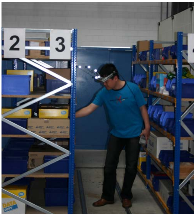
Figure 11 Pick-by-Vision including an infrared tracking system with targets fixed on the HMD
