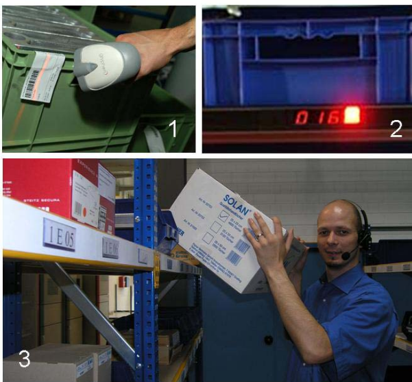
Figure 1 Usual order picking technologies: scanner (1), Pick-by-Light (2) and Pick-by-Light (3)
