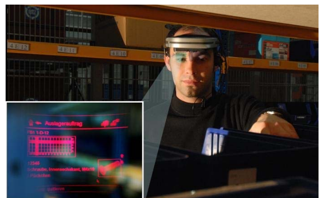
Figure 4 Used system in this set-up: a Microvision Nomad HMD, a head-set for the speech input and a possible visualization (little picture)
