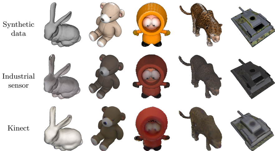
Fig. 1. SDF-2-SDF reconstructions of the proposed dataset objects. Colors vary due to difference between synthetic rendering and 3D-printed models, and camera radiometrics
