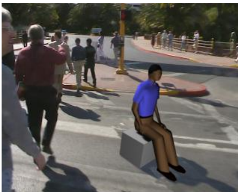
Figure 1.1: An example of visual Augmented Reality: A person is augmented to the real world. Note the shadows! (Courtesy of Loria [11])
