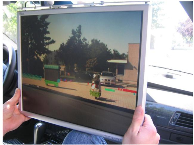
Figure 13: Snapshot of the See-Through TFT. One can see the superimposed sensor data on the garbage container and the Vespa scooter
