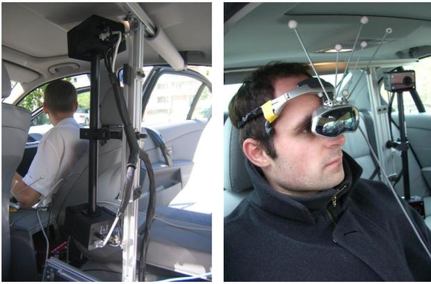
(a) Snapshot of the two tracking cameras from behind and the covered tracking volume (b) The HMD worn in the tracking volume. The tracking cameras (back right) can see the markers
