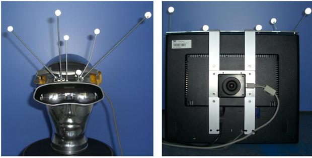
(a) HMD (Sony Glasstron PLM-S700) used for visualization worn by an artificial head (b) Backside of the 19" TFT video see-through display with an attached FireWire camera at the center
