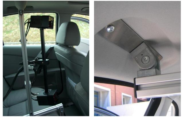
(a) Overview of the mount for the tracking system (b) Left side handhold mount for the tracking system
