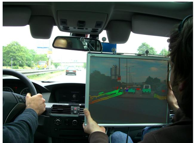
Figure 11: The TFT held into the tracking volume while driving. One can see the laser-scanner augmentation on the vehicles and the guardrail
