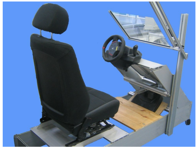
Figure 4: The driver's cockpit is build on an aluminum frame and has the same relationships as a common driver's cockpit (distances and sitting height)
