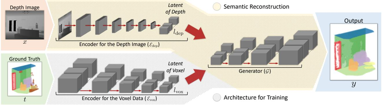
Figure 2: Deep architecture for the semantic reconstruction in Sec. 3 and for the training procedure in Sec. 4. The former is the concatenated architecture of the encoder  $\mathcal{E}_{\text{dep}}$  and the generator  $\mathcal{G}$  reconstructs from the depth image to a voxel data while the latter is the concatenated architecture of  $\mathcal{E}_{\text{vox}}$  and  $\mathcal{G}$  is a 3D variational auto-encoder [2] for self-reconstruction.
